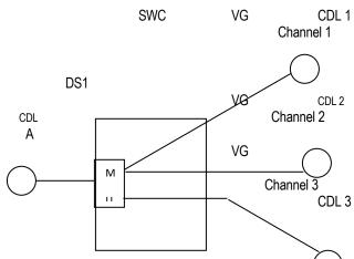
The customer requests that the voiceband circuit serving CDL 3 be (moved from channel 20 in the DS1 serving CDL A to Channel 3 in the same DS1. No NRCs apply for this request.
