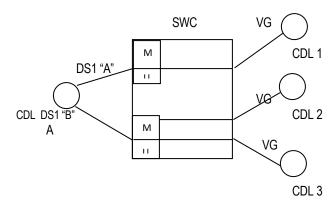
The customer requests that the voiceband (VG) circuit serving CDL 1 be moved from the DS1 "A" circuit to the DS1 "B" circuit. No NRCs apply for this request.
