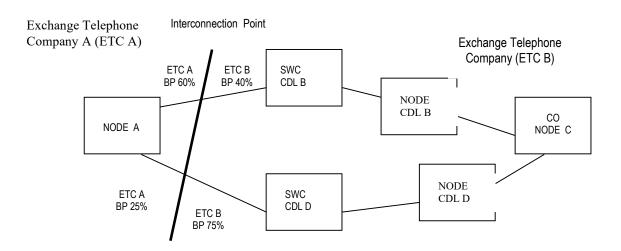
Step 1 – Calculate the total ring mileage by summing the mileage connecting all locations and devices (Node A to SWC CDL B) + (SWC CDL B to Node CDL B) + (Node CDL B to CO Node C) + (CO Node C to Node CDL D) + (Node CDL D) to SWC CDL D) + (SWC Node D to Node A), If the total ring mileage includes a fraction of a mile, the value is rounded up to the next full mile.
