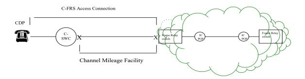
The following diagram depicts a generic view of the components of FRS Service and the manner in which the components are combined to provide a complete FRS connection.
