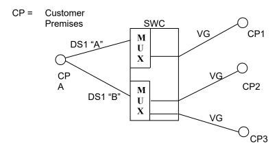
The customer request that the voiceband (VG) circuit serving customer premises 1 be moved from the DS1 "A" circuit to the DS1 "B" circuit. No NRCs apply for this request.
