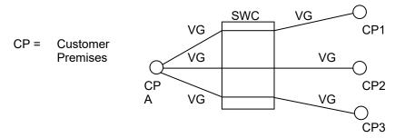
The customer request the installation of DS1 between the serving wire center (SWC) and customer premises A and DS1/Voice multiplexer in the SWC. The customer also request that the voiceband circuits serving customer premises 1,2 and 3 be "rolled over" to the new DS1. All NRCs apply for the installation of the DS1 and multiplexer. No NRCs apply for the voiceband roll overs to the new high capacity circuit.
