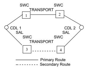
Two diverse circuits between serving wire centers. The SAL and Transport facilities must be entirely separate.
